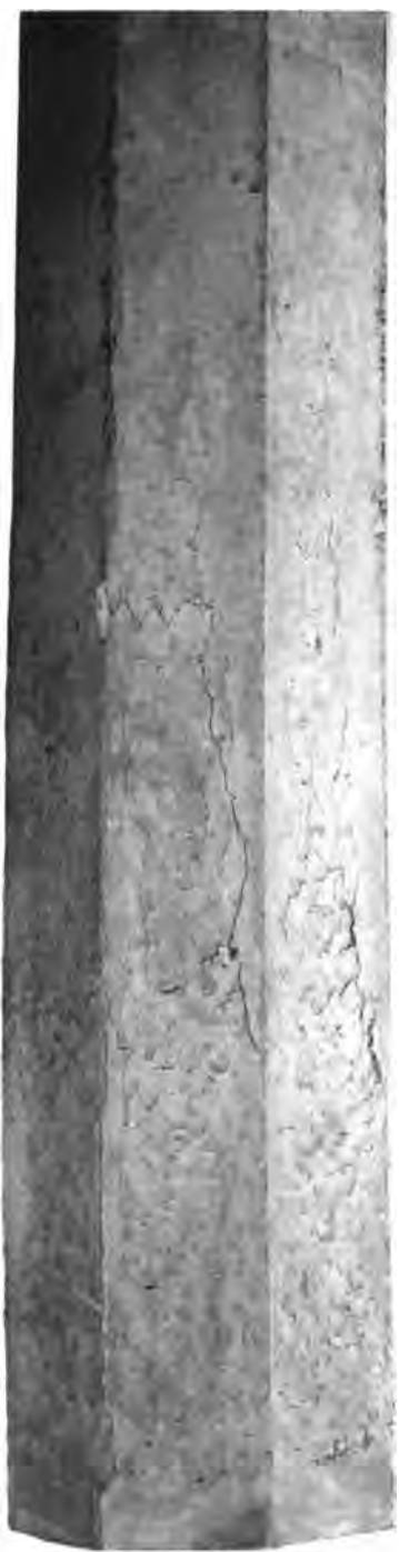
CONCRETE COLUMN NO. 1768. APPEARANCE AFTER TESTING.
